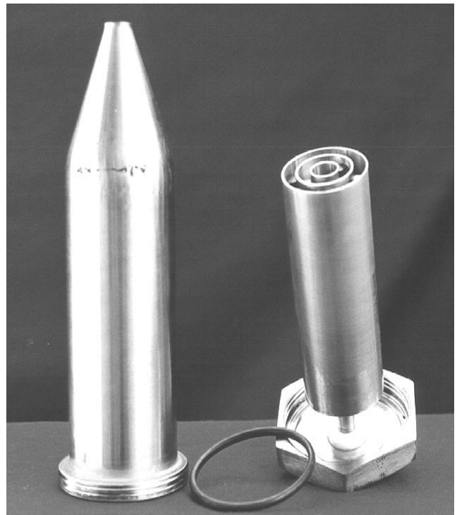
FIG 16. Cell - 4 cylinder. View of the completed cell sub-assemblies. Note that the compression fitting is missing from the top of the cone. The O-ring fits between the outer thread and the base cap
