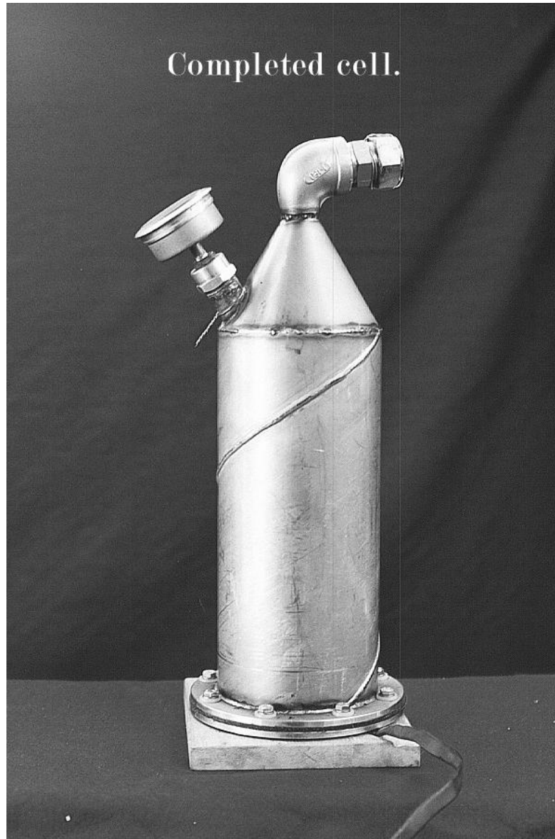
Fig. 1. - A view of "Old Trusty". A 3 year old cell that breaks most of the rules of cell design, but is still a great performer. The filling hole has a temporary pressure gauge fitted to monitor air leaks.
