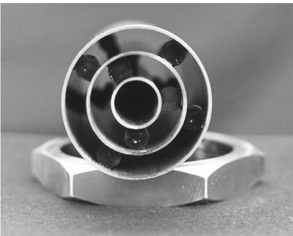
FIG 15. Cell - 4 cylinder. A view of the method for fitting the 1/2 inch long, 1/2 inch wide ebonite insulators
