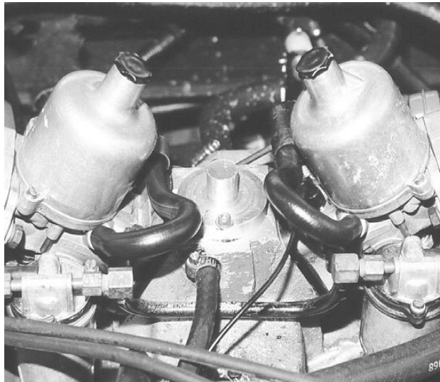
FIG 46. View of the blind plug fitted to the inlet manifold with 2 cap bolts. Plug is designed for 1 inch internal diameter hose fitting
