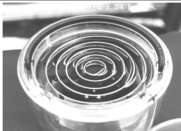
FIG 32. Stage 2 - A view after 24 Hours without power. Notice that the cell is now dead. No bubbles and no surface tension.
