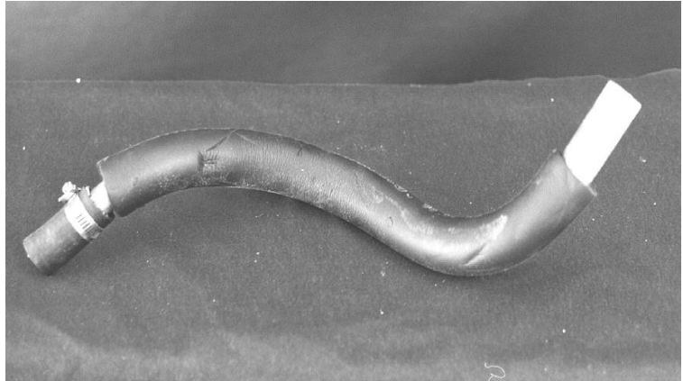
FIG 43. A view of the cell to engine connecting pipe. Notice that the blind plug end of the rubber tube does not have a hose fitting and thus would be a loose fit on the engine blind plug.
