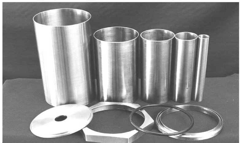
FIG 17. Cell - 5 cylinder. All major components of the cell. Note separate base plate and nut. The thread ring is still to be push fitted to the lower part of the outer cylinder.
