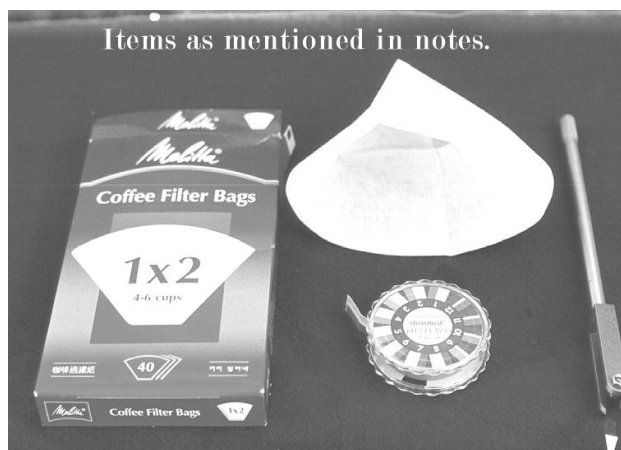
FIG 41. Left / top centre - The type of coffee filters used for filtering stream water. Bottom / Centre - Roll of Litmus paper. pH range 1-14 pH for testing the water. Right - rotating magnet for testing paramagnetism of all stainless steel components
