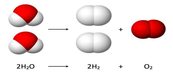
Considering the alkaline electrolyte most usual in electrolytic generation of Hydrogen and Oxygen in industrial grade PEM generators then indeed only separated H2 and O2 can be obtained with electrolyte temperature in range of 90°C, 30% KOH concentration and 1.8 Volts.
